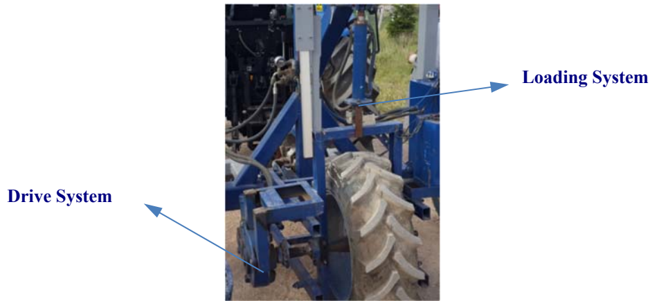
Figure 1. Single Wheel Tester Design Concept
