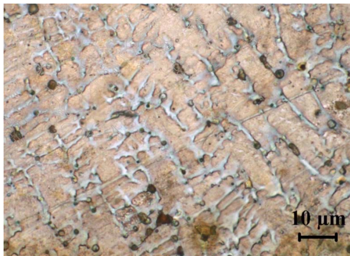
Fig. 4. Interdendritic micro-pores in the nucleus region.
